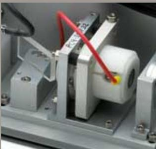
Holdoff is achieved by means of a polariser and a quarter waveplate. Horizontally polarised light incident upon the quarter waveplate is circularly polarised, upon
