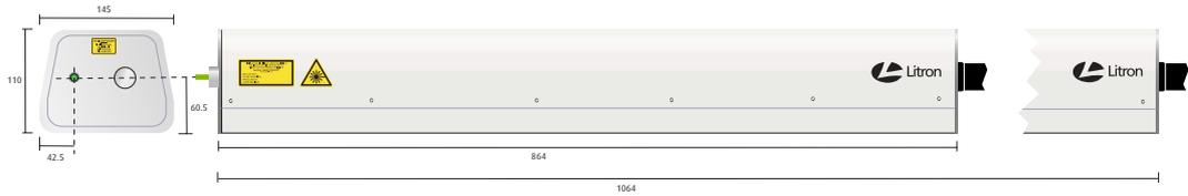
**LPY Single rail laser head arrangement**
