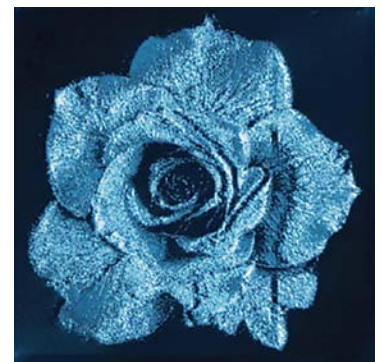
“Birefringent rose” image fabricated in bulk of quartz substrate. Dimensions 1×1 mm.
